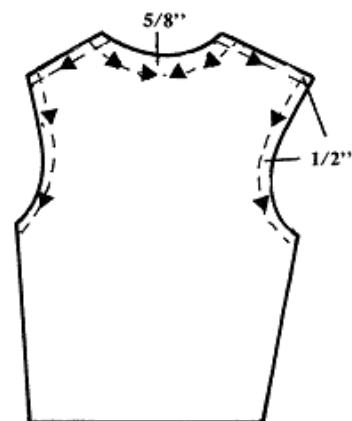
Figure 2. Stay stitch curved and biased edges to prevent stretching.
